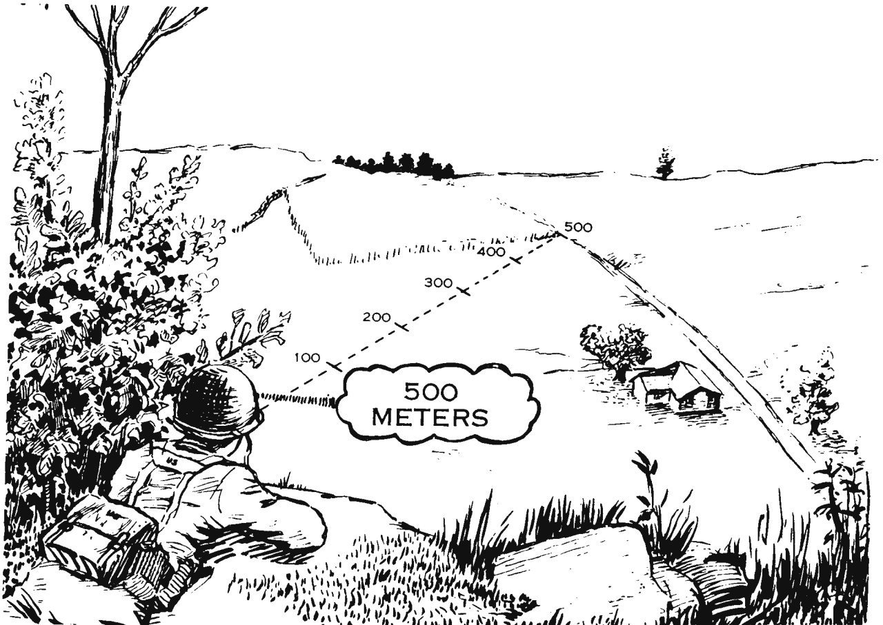
Figure 77. Applying the 100-meter unit of measure method for ranges up to 500 meters.
