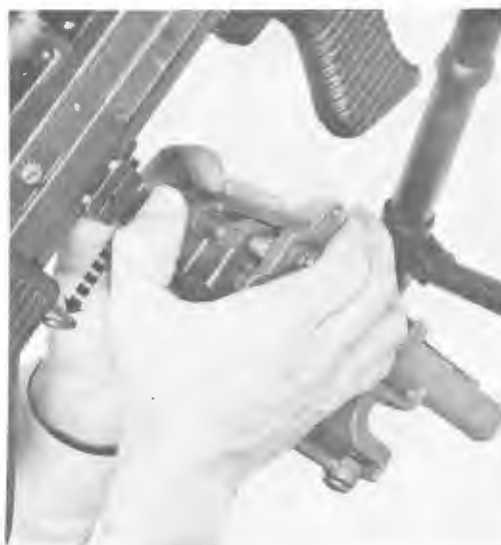
Figure 38. Removing the traversing and elevating mechanism.
