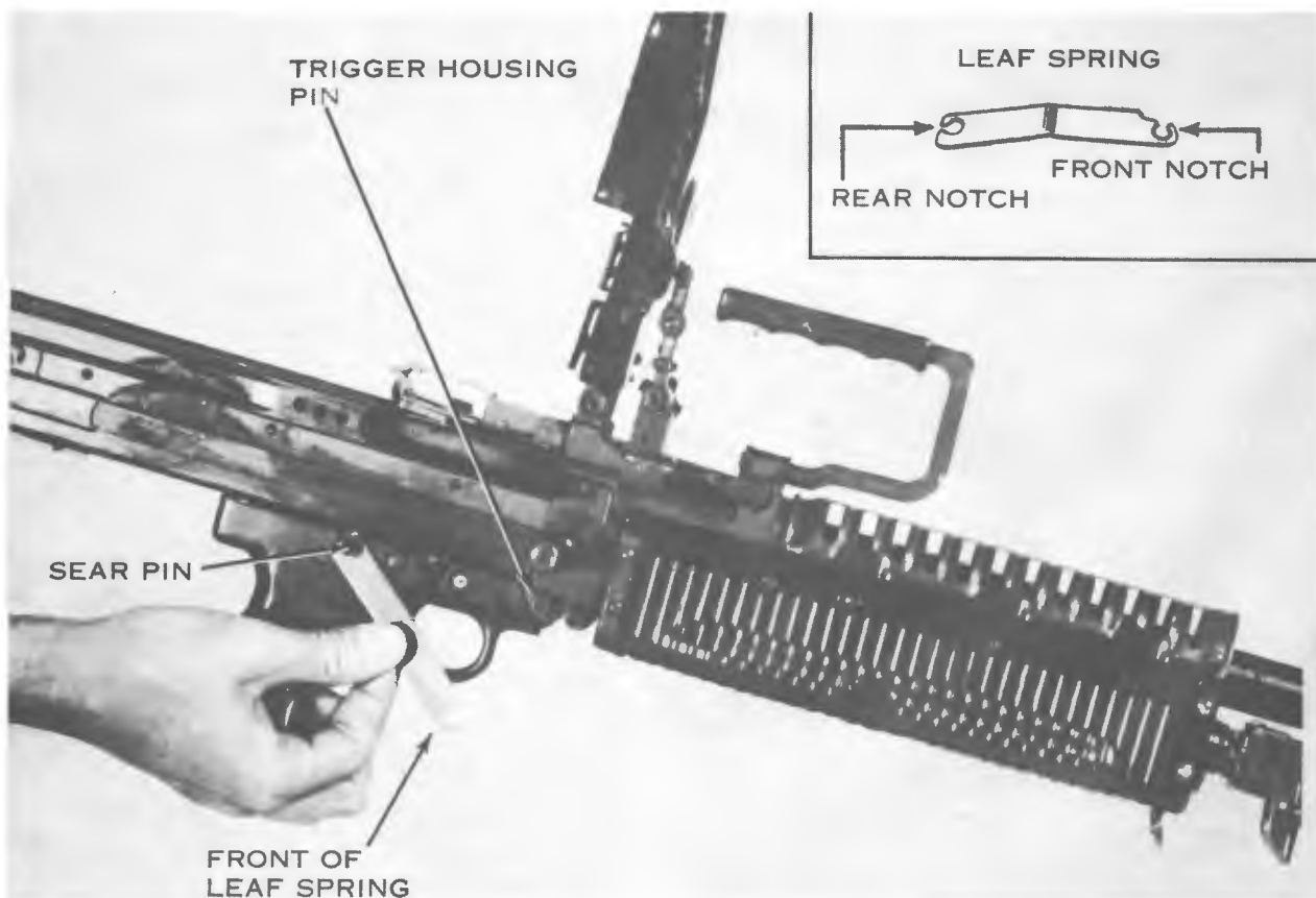
Figure 9. Removing the leaf spring.
