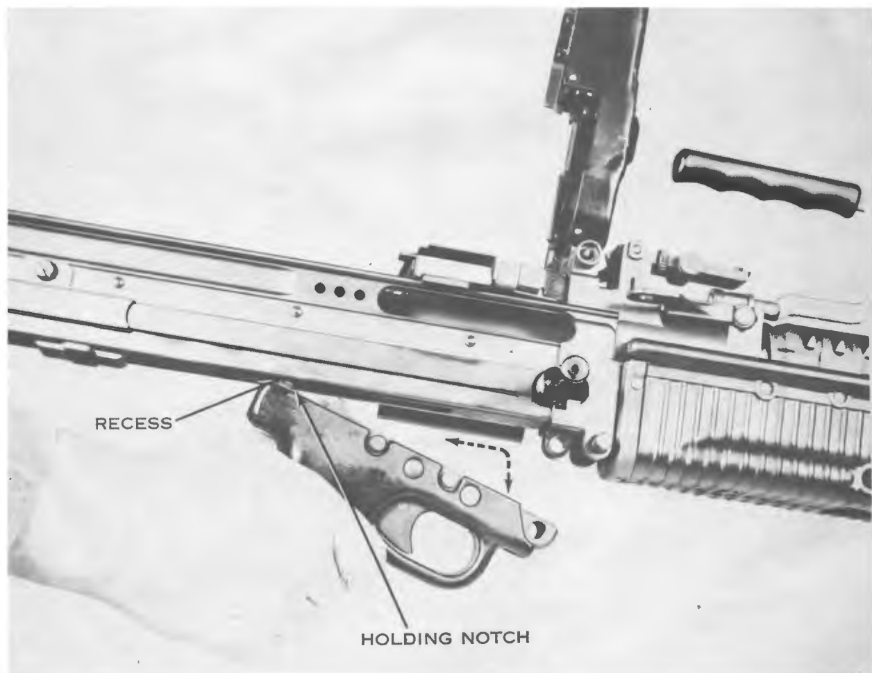
Figure 10. Removing the trigger housing group.
