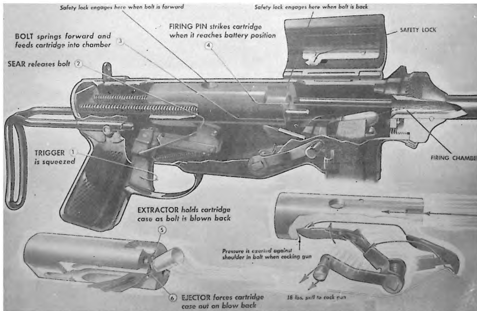
FIG. 16. Basic functioning, U.S. submachine gun, caliber .45, M3.
