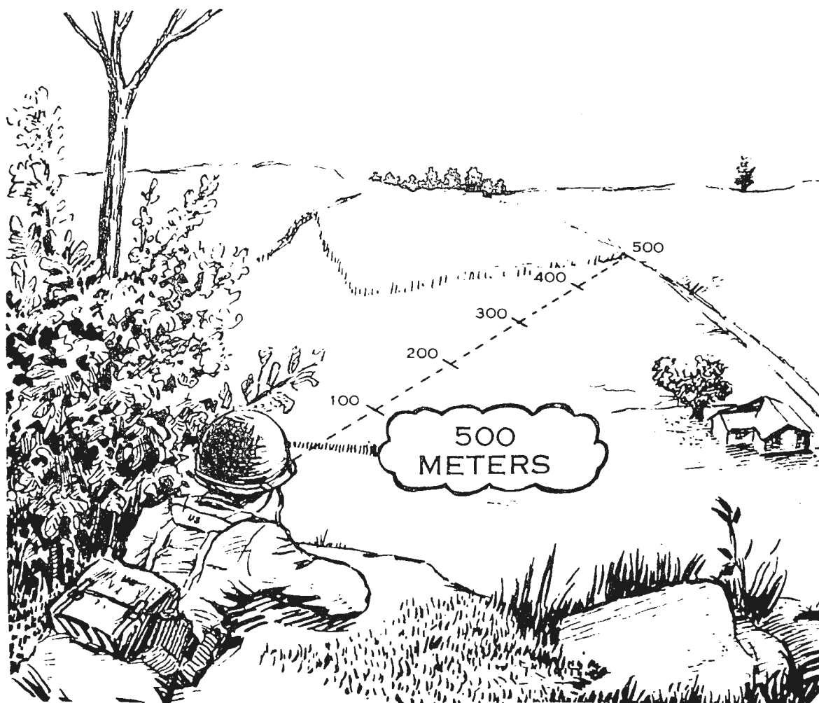
FIGURE 75 APPLYING THE 100-METER UNIT OF MEASURE METHOD FOR RANGES UP TO 500 METERS
