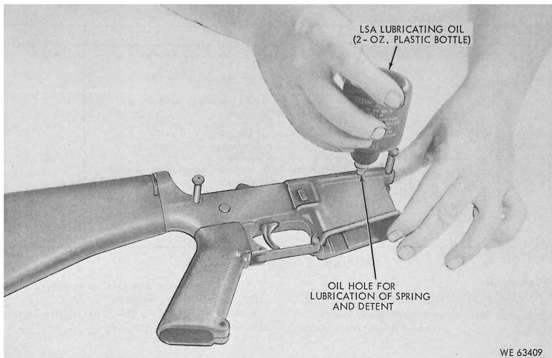
Figure 2-10. Oiling detent and spring.
